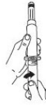
2. Thread vial into injector 3 half turns, or until vial is pierced by metal cannula.* DO NOT PUSH VIAL INTO INJECTOR; THIS MAY CAUSE MISALIGNMENT.
