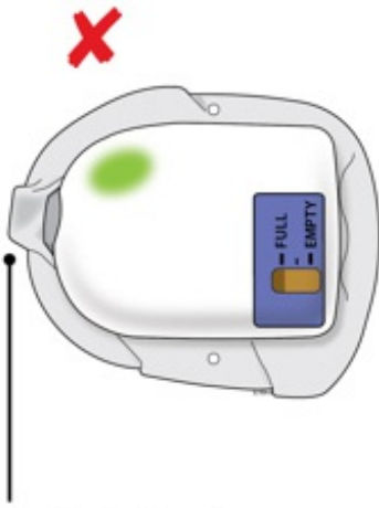
Wrinkled adhesive near cannula window
