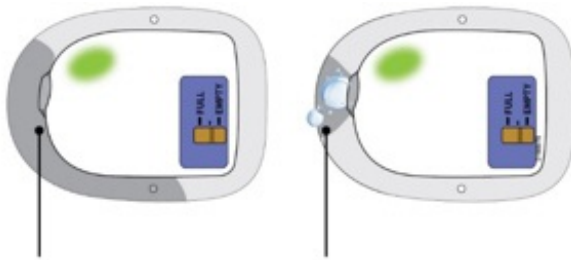
Dripping fluid from on-body injector
