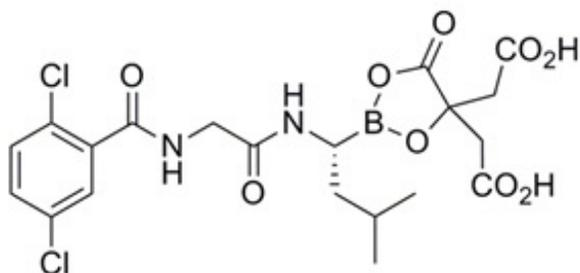
The molecular formula for ixazomib citrate is  $C_{20}H_{23}BCl_2N_2O_9$  and its molecular weight is 517.12. Ixazomib citrate has one chiral center and is the R-stereoisomer. The solubility of ixazomib citrate in 0.1N HCl (pH 1.2) at 37°C is 0.61 mg/mL (reported as ixazomib). The solubility increases as the pH increases.
