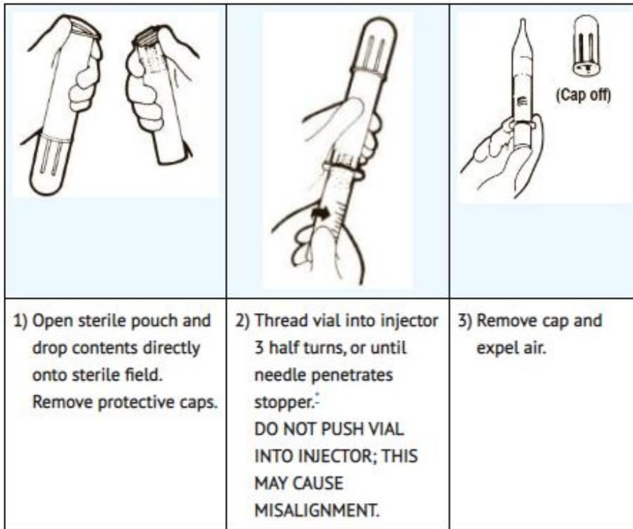
⚠ CAUTION: IMPROPER ENGAGING MAY CAUSE GLASS BREAKAGE AND SUBSEQUENT INJURY.
