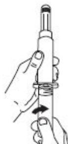
2. Thread vial into injector 3 half turns, or until stopper is pierced by metal cannula.* DO NOT PUSH VIAL INTO INJECTOR; THIS MAY CAUSE MISALIGNMENT.
