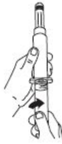
2. Thread vial into injector 3 half turns, or until vial is pierced by metal cannula.* DO NOT PUSH VIAL INTO INJECTOR; THIS MAY CAUSE MISALIGNMENT.
