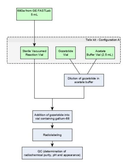
Note: Ga 68 from GE FASTlab is aseptically transferred into the Sterile Vacuumed Reaction Vial.
