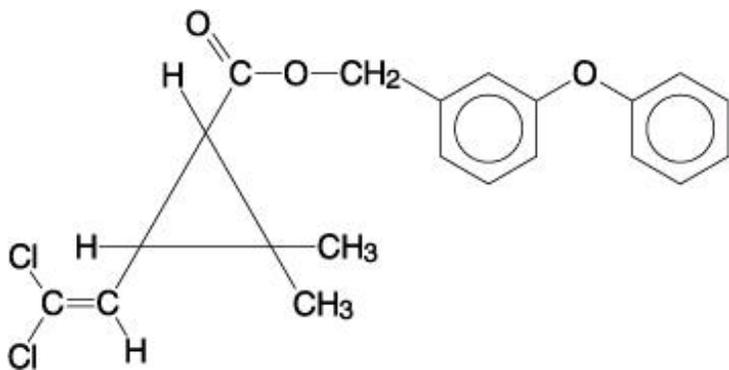
**Chemical Name:** The permethrin used is an approximate 1:3 mixture of the cis and trans isomers of the pyrethroid 3-(2,2-dichloroethenyl)- 2,2-dimethylcyclopropanecarboxylic acid, (3-phenoxyphenyl) methyl ester. Permethrin has a molecular formula of C<sub>21</sub>H<sub>20</sub>Cl<sub>2</sub>O<sub>3</sub> and a molecular weight of 391.29. It is a yellow to light orange-brown, low melting solid or viscous liquid.
