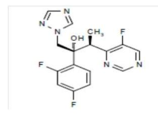
Voriconazole is designated chemically as  $(\alpha R,\beta S)-\alpha-(2,4-difluorophenyl)-5-$  fluoro- $\beta$ -methyl- $\alpha$ -(1H-1,2,4-traizol-l-ylmethyl)-4-pyrimidineethanol with an empirical formula of C16H14F3N5O and a molecular weight of 349.31 g/mole.
