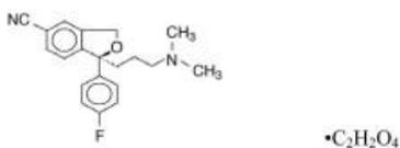
The molecular formula is  $\text{C}_{20}\text{H}_{21}\text{FN}_2\text{O} \cdot \text{C}_2\text{H}_2\text{O}_4$  and the molecular weight is 414.43.
