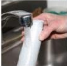
Figure E: If the can seems warm or the foam is runny, run the can under cold water.
