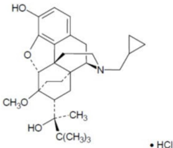
Buprenorphine HCl has the molecular formula  $C_{29}H_{41}NO_4 \cdot HCl$  and the molecular weight is 504.10. It is a white or off-white crystalline powder, sparingly soluble in water, freely soluble in methanol, soluble in alcohol, and practically insoluble in cyclohexane.
