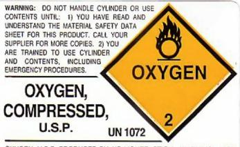
OXYGEN, U.S.P. PRODUCED BY AIR LIQUEFACTION, WARNING: HIGH PRESSURE OXIDIZING GAS. VIGOROUSLY ACCELERATES COMBUSTION. Secure cylinder in storage and use. Keep oil and grease away. No smoking in cylinder area. Open valve slowly. Use only with equipment cleaned for oxygen service and rated for cylinder pressure. Close valve after each use and when empty. Use in accordance with Material Safety Data Sheet.
