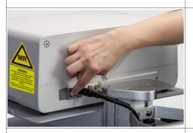
**3. Press** the Black Rocker Power Switch, located on the back of each Console. to the right (ON position) to power on **both** Consoles.
