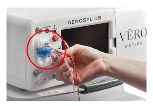
3. Push and twist the short Y-end of the Manual Ventilation Line (clear) to the Manual
