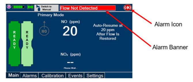
The alarm banner contains a drop-down menu containing a list of all alarms should there be multiple activated. The alarm icon is always present on the top right of the screen and tapping the icon will pre-silence or silence alarms. Refer the table below for descriptions of each alarm status:
