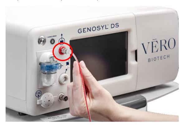
2. <u>Push</u> and <u>twist</u> the short Y-end of the Sample Line (blue) to the Gas Sample Port on the front of the Water Trap, attached to the top Console.
