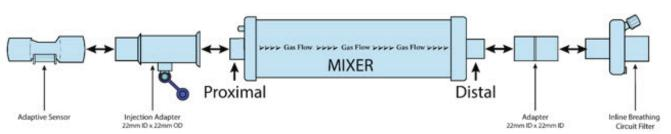
Figure 9: GENOSYL DS Mixer Assembly with Adaptive Sensor
