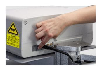
**12**<u>Press</u> the Black Rocker Power Switch to the "OFF" position.
