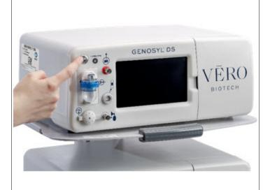
4. Press the Silver Power Button. located at the top left corner on the front panel of each Console, to turn on the display screens on both Consoles. The display screen will illuminate. and the Consoles will beep, indicating the power is on.
