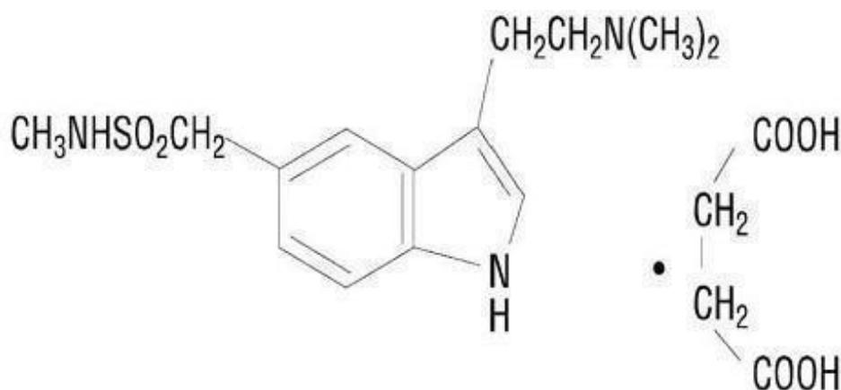
The empirical formula is C<sub>14</sub>H<sub>21</sub>N<sub>3</sub>O<sub>2</sub>S•C<sub>4</sub>H<sub>6</sub>O<sub>4</sub>, representing a molecular weight of 413.5. Sumatriptan succinate is a white to off-white powder that is readily soluble in water and in saline.
