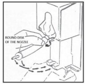
4. Before closing the cover, check to make sure the round disk of the nozzle is firmly in place at the bottom of the lower locator.
