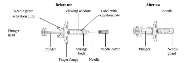
Grasp the syringe body to remove the pre-filled syringe from its tray. Do not 1 grab the pre-filled syringe by the plunger.
