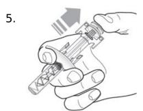
After injection, maintain pressure on the plunger head and remove the needle from the skin. Release pressure on the plunger head to allow the needle guard to cover the needle. Do not re-cap the pre-filled syringe. Discard the used syringe into a sharps container.
