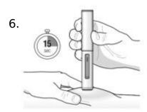
Hold down firmly for about 15 seconds. You will hear a second 'click', this tells you the injection has finished. The orange plunger will fill the viewing window.
