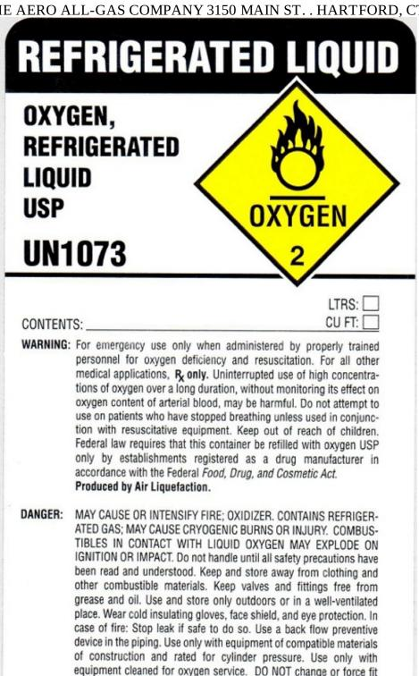
connections. Avoid spills. Do not walk on or roll equipment over spills. Close valve after each use and when empty. Always keep container in unright position. Dood and follow the Cafety Date Cha
