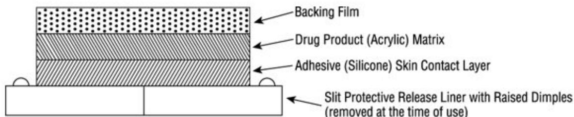
**Figure 1: Cross Section of the Rivastigmine Transdermal System**
