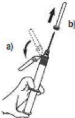
**DO NOT PUSH VIAL INTO INJECTOR; THIS MAY CAUSE MISALIGNMENT OF THE INJECTOR NEEDLE.**
