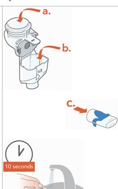
Clean all Handset parts by adding a few drops of clear liquid dish soap and warm tap water to a clean tub or bowl. Cover the Handset parts in the warm soapy water and soak for 5 minutes, shaking them periodically. Then rinse them thoroughly under warm running tap water.
