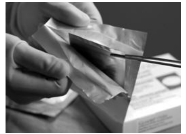
Figure 4: To open the inner pouch, gently hold the crimped edge and cut in an arc-like fashion around the wafer.
