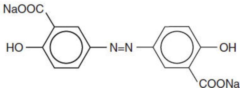
Olsalazine sodium is a yellow crystalline powder, which melts with decomposition at 240°C. It is the sodium salt of a weak acid, soluble in water and DMSO, and practically insoluble in ethanol, chloroform, and ether. Olsalazine sodium has acceptable stability under acidic or basic conditions.
