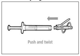
Push and twist the injection needle clockwise on to the syringe until it is fully attached.
