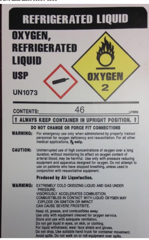
Cylinder temperature should not exceed 52°C (125°F).
