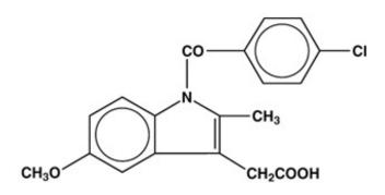
The molecular formula is  $C_{19}H_{16}CINO_4$  and the molecular weight is 357.79. Indomethacin, USP is practically insoluble in water and sparingly soluble in alcohol. It has a pKa of 4.5 and is stable in neutral or slightly acidic media and decomposes in strong alkali.
