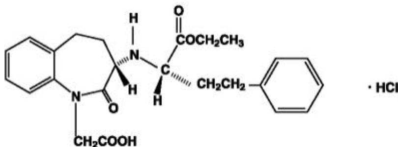
Its empirical formula is  $C_{24}H_{28}N_2O_5 \cdot HCl$ , and its molecular weight is 460.96.
