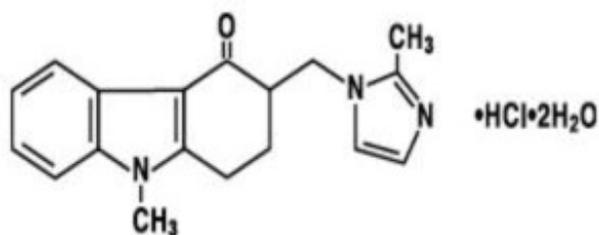
The empirical formula is C<sub>18</sub>H<sub>19</sub>N<sub>3</sub>O·HCl·2H<sub>2</sub>O, representing a molecular weight of 365.9 g/mol.
