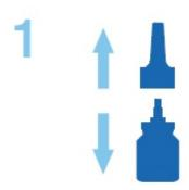
Remove spray nozzle by grasping at base and pulling up.
