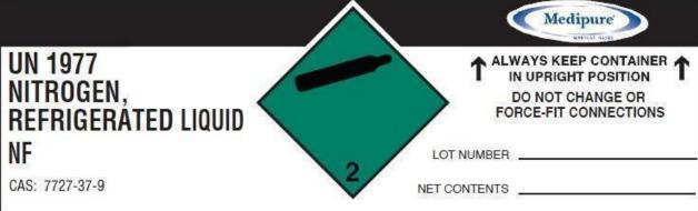
WARNING! EXTREMELY COLD LIQUID AND GAS UNDER PRESSURE. CAN CAUSE RAPID SUFFOCATION. CAN CAUSE SEVERE FROSTBITE. MAY CAUSE DIZZINESS AND DROWSINESS.
