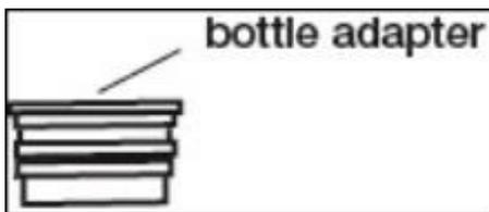
Once the bottle adapter is installed, it cannot be removed. **See Figure D**
