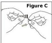
**STEP 3.** Pick up the Needle Assembly. Grab the paper tab and peel off the paper cover (lid) from the bottom of the needle assembly (Figure C).
