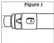
Then – holding the syringe as shown in Figure I, **slowly turn the plunger rod clockwise** (like tightening a screw – see arrow in Figure I) until the correct dose number appears **in the center of the window** (Figure J).
