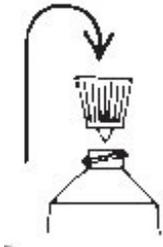
2. Use the pointed tip on the top of the cap to puncture the seal on the tube.
