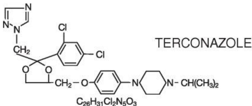
Terconazole, a triazole derivative, is a white to almost white powder with a molecular weight of 532.47. It is insoluble in water; sparingly soluble in ethanol; and soluble in butanol.
