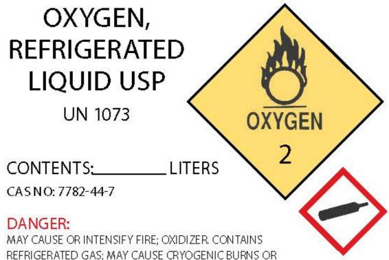
INJURY. COMBUSTIBLES IN CONTACT WITH LIQUID OXYGEN MAY EXPLODE ON IGNITION OR IMPACT.
