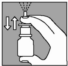
The pump is now ready for use. If the pump is not used for 7 days, prime until a fine spray appears.
