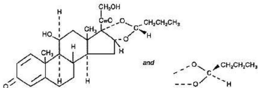
Budesonide is a white to off-white, tasteless, odorless powder which is practically insoluble in water and in heptane, sparingly soluble in ethanol, and freely soluble in chloroform. Its partition coefficient between octanol and water at pH 7.4 is  $1.6 \times 10^3$ .
