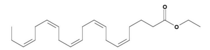
The empirical formula of DHA ethyl ester is  $C_{24}H_{36}O_2$ , and the molecular weight of DHA ethyl ester is 356.55. The structural formula of DHA ethyl ester is:
