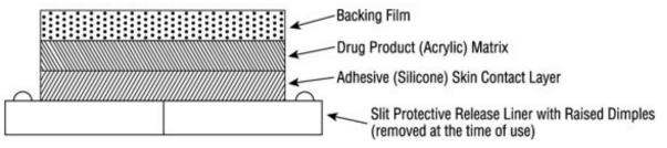
Figure 1: Cross Section of the Rivastigmine Transdermal System
