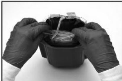
**7** Press the satellite containers (and inserts if used) down into the liner before pressing down the primary container.
