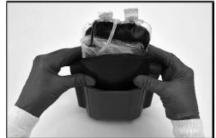
**6** Hold the bundle and insert into the centrifuge cup.
