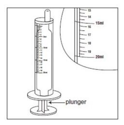
**Step 5.** Insert the syringe into the upright bottle and push the plunger all the way down. **See Figure F**
