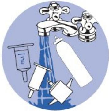
**7** After each use, applicator parts should be pulled apart for thorough cleaning with warm water. Since some foam will appear under the cap, the cap and underlying tip should be pulled apart and rinsed to help prevent build-up of foam and possible blockage.
