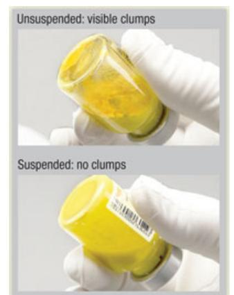
Figure 3: Check for unsuspended powder and repeat tapping if needed.
