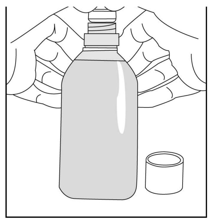
4. Replace the cap to be sure that the adapter has been fully forced into the neck of the bottle.
